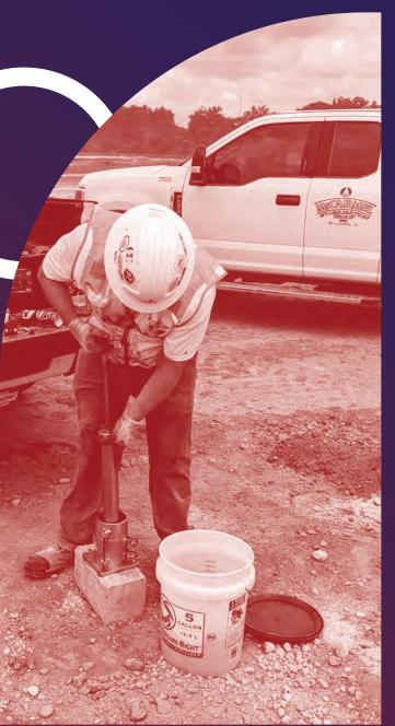
The labs also performed untreated and treated Proctors with bulk samples taken in the field and with the chemicals used on site to establish what the untreated and treated optimum moisture contents were. Field strength specimens were also molded at each location for each chemical treatment to estimate how much strength would be gained by modifying the soil. The labs did a variety of field-molded strength specimens for testing at various curing periods.
